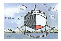
boat) out of the water. The hydrofoil stays in the water, holding the boat up with struts.
