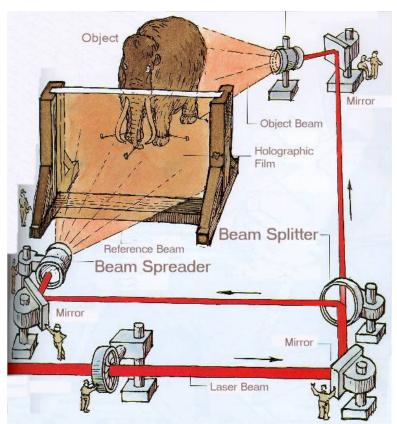
reflects off the object onto the holographic film. Therefore we now have laser light shining on both sides of the holographic film, and this by exposing the film to laser light, we can produce a three-dimensional image of the object on the film.
