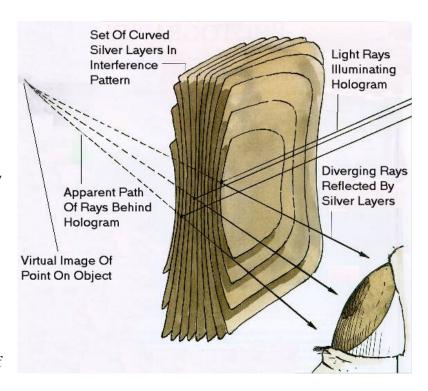
the original object at different angles. Therefore with the multiple layers in the holographic film, we are able to effectively preserve what the object looked like from many different angles.
